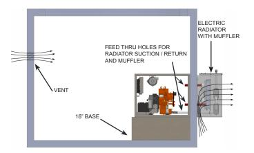
This installation configuration has the electric radiator and silencer / muffler assembly external to the shelter. This installation has popularity in very cold climates where there is the need to reduce the amount of low temperature air moving through the shelter. In this configuration only the combustion air and a very small amount cooling air is required from the vent on the wall.
