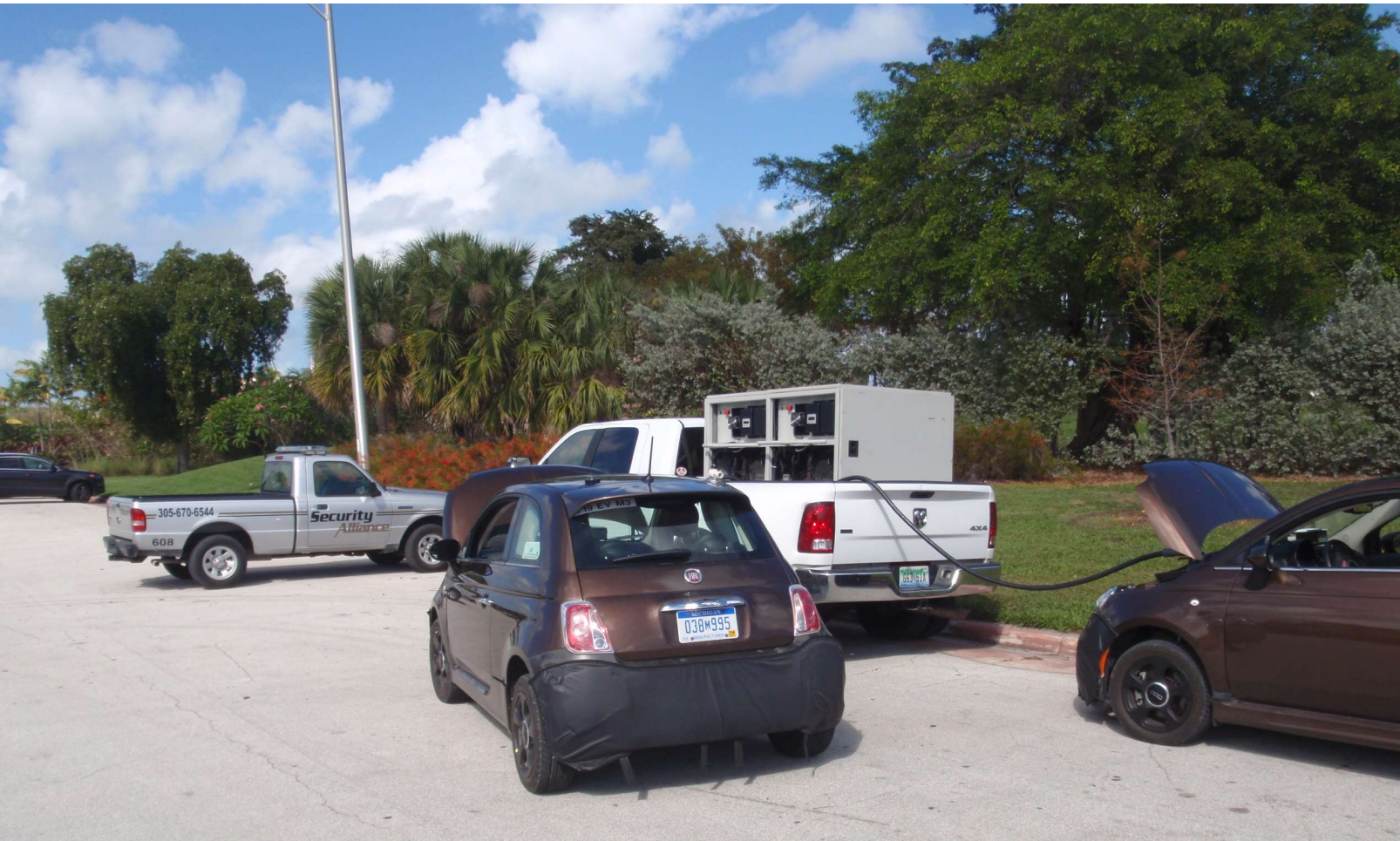
Two Polar 27 kW DC generators mounted on the back of a pickup truck charging 2 EVs during their field trails
