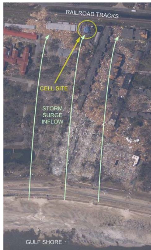
Fig. 6.21 Aerial picture showing the storm surge inflow near the cell site at the water tower [6]
