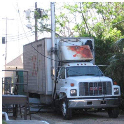
Fig. 6.66. COW behind BellSouth Gulfport CO
