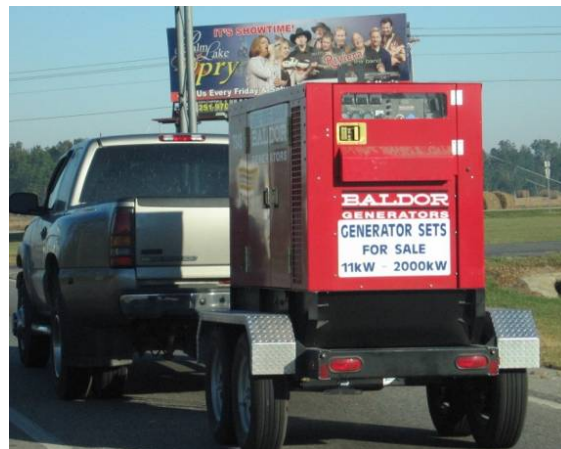
Fig. 2.17. Trailer genset being transported
